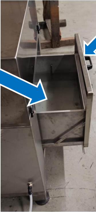
Recirculation solvent reservoir with the capacity of 80 litres
